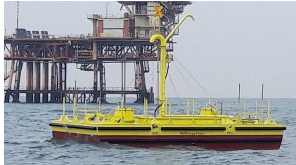
ISWEC pilot version linked to Ravenna's O&G platform
